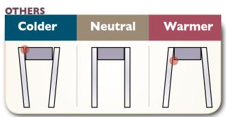
With conventional aluminum spacers, the sealant flexes which can lead to sealant failure and loss of insulating ability.
