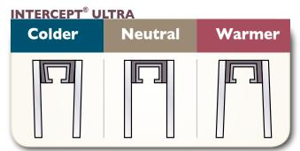
Intercept<sup>®</sup> Ultra spacers flex instead of the sealant during temperature changes so it resists spacer movement and seal failure.
