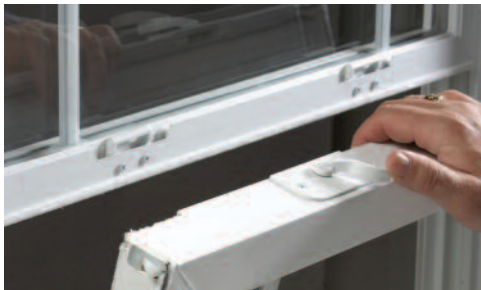
Low profile locking hardware serves a dual function. The cam action lock secures the window closed and the hidden "clean" mechanism releases the sash for tilt-in cleaning.
