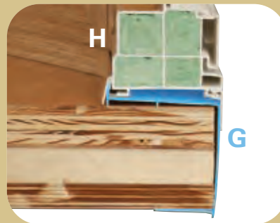
G. Exclusive welded sill pan (highlighted in blue) eliminates water penetration. The unique design provides a built-in weep system and a smooth finish on the exterior surface of the seat board. H. All window and mull cavities are insulated completely with Comfort-Foam™ for maximum energy efficiency.
