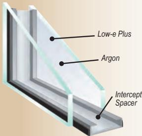
This window is Energy Star qualified in North, North-Central, & South-Central zones. Upgrade of SOLAR LOW-E qualifies window in South zone and provides: U-factor: 0.29, SHGC: 0.22, Visible Transmittance: 0.51
