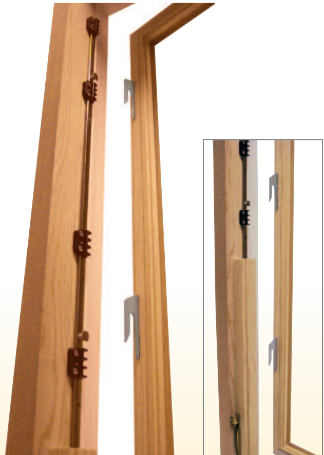
The multi-point lockbar features adjustable self-locating lock points for maximum pull-in capability of the sash against the weather stripping to prevent water and air infiltration.
